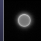
hollow fluorescent 15-micron sphere, manually captured Z-stack, 1-micron increments, 40×/1.3NA oil objective
