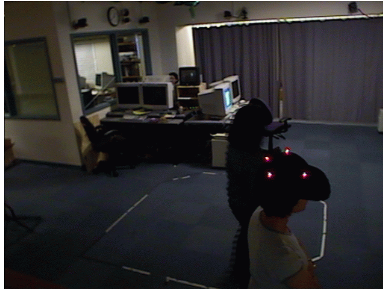
Figure 2.11: A video frame from a camera showing a person wearing a hat mounted with bright red LEDs.
