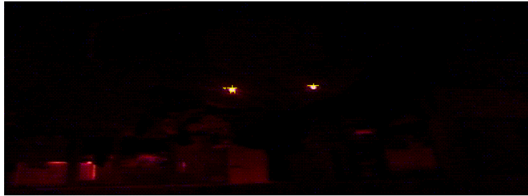
Figure 2.2: A video frame from a camera with the detected LEDs marked with yellow crosses. The background appears to be very dark compared to the LEDs because we have put a red filter in front of each camera lens so that much of the light outside the passband of the LED is attenuated. The use of only an absolute threshold is not flexible, and the use of only a relative threshold can result in a very low threshold setting that is not robust to noise.
