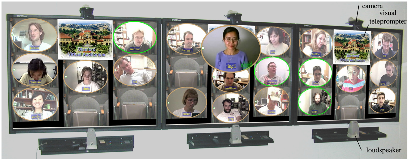
Figure 1. The Virtual Auditorium display wall. This wall can display 24 students and the instructor can move students to different seats. Videos are elliptically shaped to provide a common background for all students. A student's voice is rendered from the loudspeaker closest to his image and his instantaneous audio amplitude is displayed next to his name. The audio localization and amplitude display allow the instructor to easily identify the speaker. Directly below the cameras are regions called the visual teleprompters that show visual aids or students in directed gaze mode.
