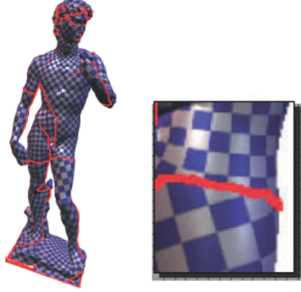
Figure 1: Edge discontinuities common in mapping algorithms that cut the mesh first and then recompute the metric.
