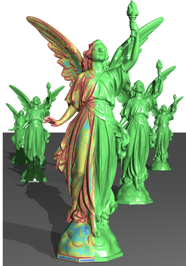
Figure 1: The Stanford Lucy, consisting of 14 million points, is reconstructed as an MPU implicit with a 0.01% max-norm approximation accuracy; the left part of the model is colored according to the subdivision level which increases from blue to red. The four models in the back are reconstructed from the point set with increasing approximation error.
