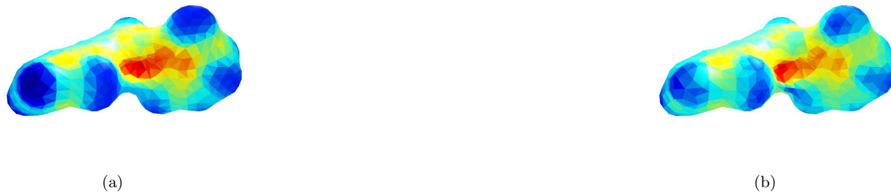
Figure 4: Connolly function (C - 2\pi)/(\pi \cdot r) (left) versus mean curvature (right) on a molecular surface. Color scales are mapped from -0.746 \dots 0.466 (left) and from -0.877 \dots 0.663 .
