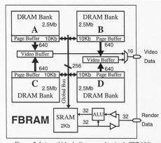
Figure 2. Internal block diagram of a single FBRAM.
