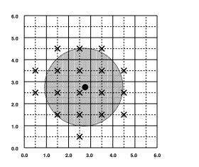
Figure 3.3. Rasterization of antialiased wide points. The black dot indicates the point to be rasterized. The shaded region has the specified width. The X marks indicate those fragment centers produced by rasterization. A fragment's computed coverage value is based on the portion of the shaded region that covers the corresponding fragment square. Solid lines lie on integer coordinates.
