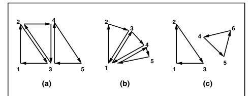
Figure 2.4. (a) A triangle strip. (b) A triangle fan. (c) Independent triangles. The numbers give the sequencing of the vertices between **Begin** and **End**. Note that in (a) and (b) triangle edge ordering is determined by the first triangle, while in (c) the order of each triangle's edges is independent of the other triangles.
