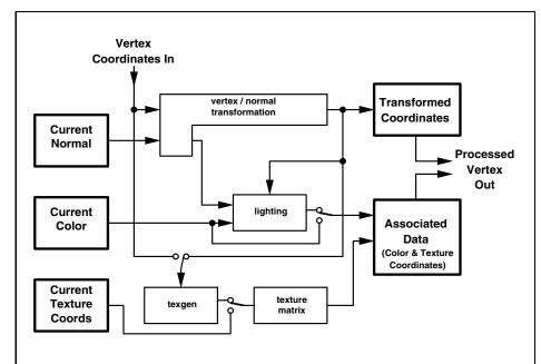
Figure 2.2. Association of current values with a vertex. The heavy lined boxes represent  $\mathrm{GL}$  state.
