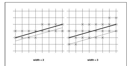
Figure 3.5. Rasterization of non-antialiased wide lines. x-major line segments are shown. The heavy line segment is the one specified to be rasterized; the light segment is the offset segment used for rasterization. x marks indicate the fragment centers produced by rasterization.
