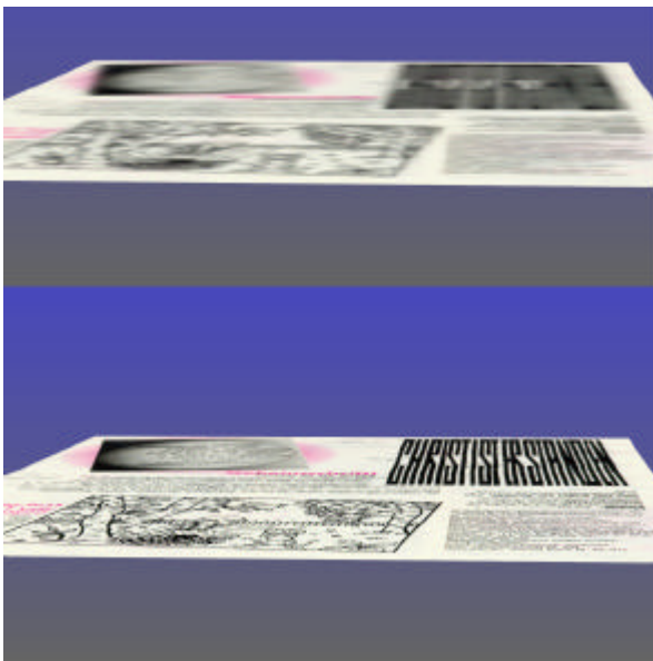
Fig. 2: Top: solving the puzzle with standard mip-mapping, as applied in cheap but also in very expensive systems. Bottom: solving the puzzle with footprint-assembly
