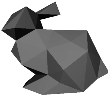
Figure 10: An approximation using only 100 triangles (generated in 15 seconds).
