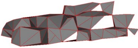
Figure 15: Uniform Vertex Clustering. 262 face approximation ( 11 \times 4 \times 4 grid). Indiscriminate joining destroys approximation quality.
